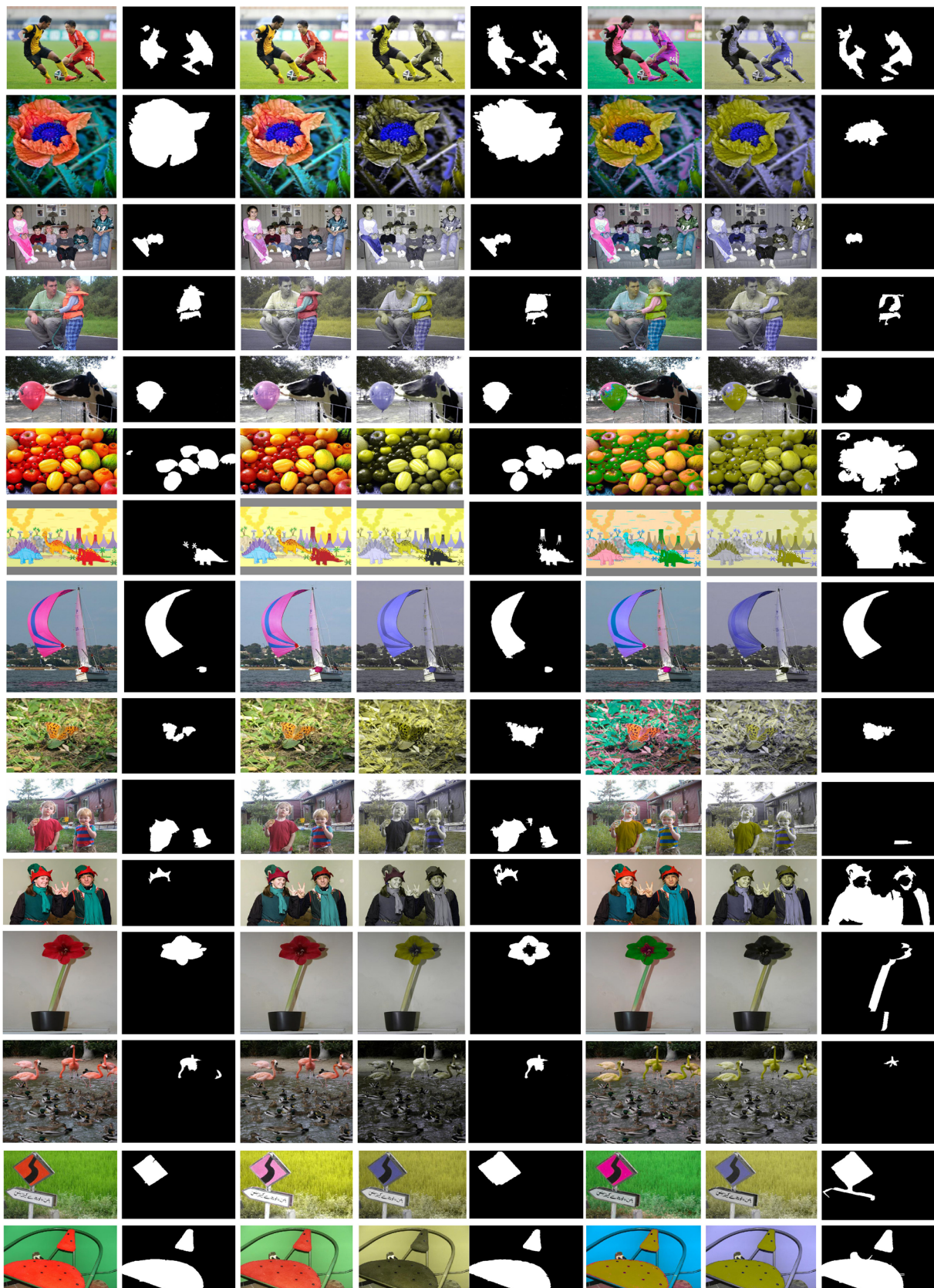
Fig. 10 For the protanopia image, compare our method with Huang's color correction algorithm.
